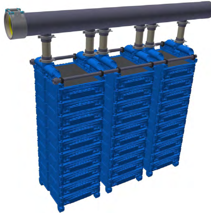
Single header pipe for each Tower-Rack line with intermediate hose connection to single towers for retrofit/rehabilitation/replacement projects (larger/existing tolerances can be compensated) Typically used for drinking water applications with high flux of up to 1,500 LMH
