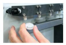
The EZ SDI<sup>™</sup> uses standard disposable filter cartridges.
