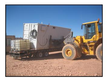
The systems are totally contained in a 20 foot intermodal shipping containers. All components of the treatment systems are mounted inside the containers. Portability of the systems allows them to be easily moved when the associated drilling equipment is moved to a new well site.
