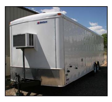
The system is mounted inside a 28 foot cargo trailer. It is totally self-contained and equipped with air conditioning to prolong the component life in a hot, humid environment. The system operates from a single 460 volt AC power source.
