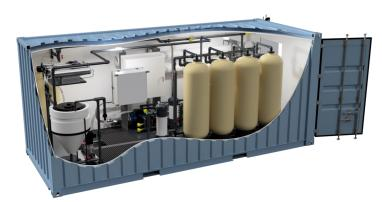
**Construction** — All of the PureBox™ systems are constructed of new, industrial quality materials. Piping, vessels, and other system components are supported inside the container with fiberglass structural members.
